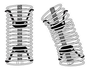
This tool is designed to handle springs up to 5-5/8 in. outside diameter and wire diameter of a maximum of 3/4 in
