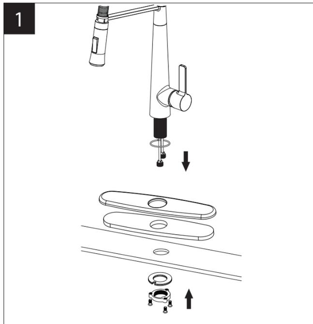
1. Position the faucet in order on the counter top as shown. Don't forget the O-ring. Assemble gasket assembly and lock nut to faucet threaded sleeve by hand and tighten the screws with screwdriver.
