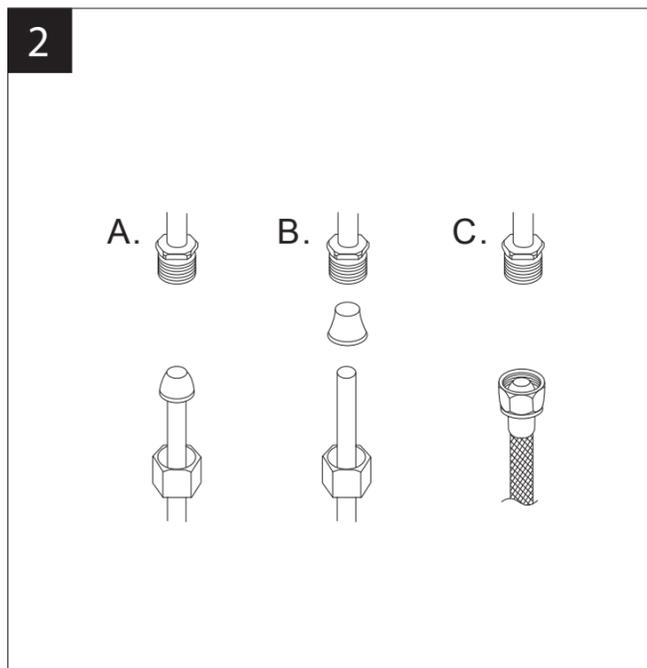
3. Connect to water supply lines with either:
