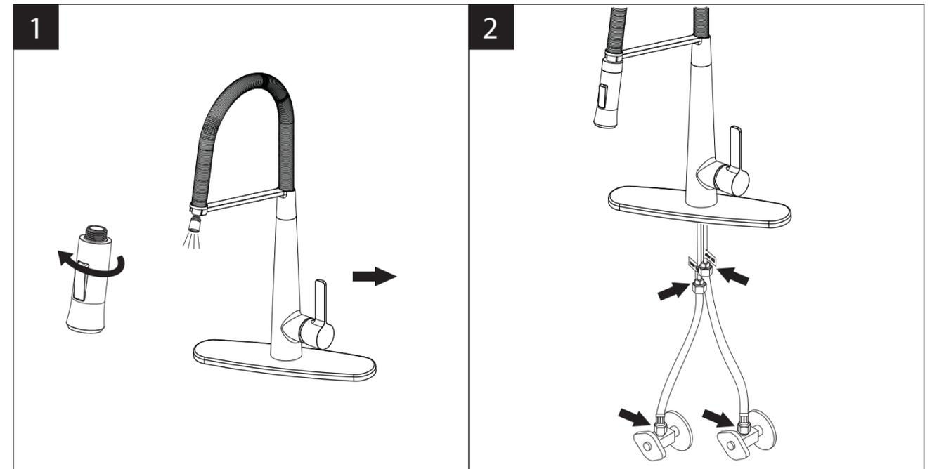
1. Remove the shower by hand. Turn the faucet handle all the way on, turn on hot and cold water supply and flush water lines for one minute. Reinstall shower by hand.
