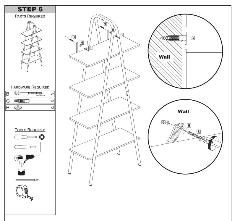
**WARNING:** Check for pipes and electrical wiring before drilling.
