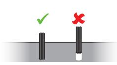
Install wood dowels by gently tapping them into the designated hole using a rubber mallet.
