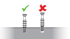
Use a screwdriver to tighten the cam screw until the shoulder is flush with the panel. Do not overtighten or under-tighten.
