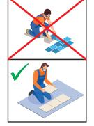
Assemble on a soft, flat, clean, and drv surface.
