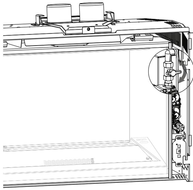
The shut-off valve is in the OFF position when the handle is horizontal (see illustration).
