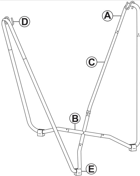
1. Carefully snap or slide Foot (E) onto the curved edge of Leg (C) as shown.
