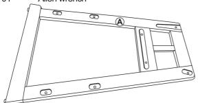
1. Place side A on flat surface with slot facing up.
