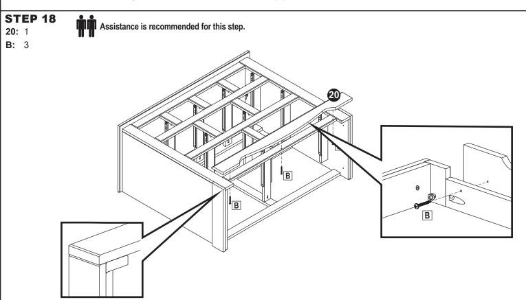
Align Front Trim Board (20) with the bottom, front of the unit. To ensure the trim board remains flush with the unit, have an assistant hold it firmly in place while the hardware is secured. From the backside of the bottom horizontal frame, secure the trim board using three M4.5x28mm Pan Screws (B).
