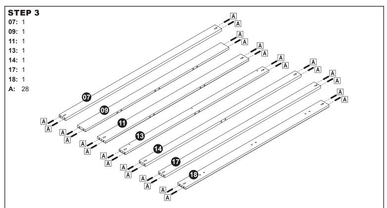
Install two Wood Dowels (A) into each end of the these components: Front Top Horizontal Face Frame (07), Top Drawer Horizontal Face Frame (09), Bottom Drawer Horizontal Face Frame (11), Bottom Horizontal Frame (13), Back Bottom Horizontal Support (14), Back Center Horizontal Support (17), and Back Top Horizontal Support (18). Set components aside, label if necessary.
