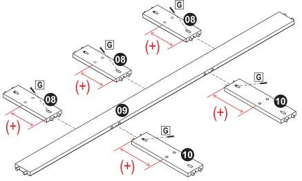
Installation direction is very important in this step. Identify the longer gap between the dowel mounting holes and the edge of Top Drawer Vertical Face Frames (08) and Middle Drawer Vertical Face Frames (10).
