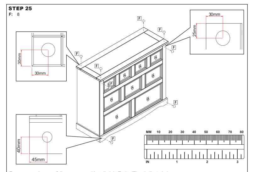
For even spacing, carefully measure and install eight Tacks (F) as indicated above.
