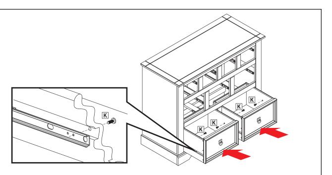
Working one drawer at a time, extend the drawer slides out from the bottom row cabinet. Align the first small hole on the drawer slide with the pre-drilled hole on the front of the drawer sides. From the inside of the drawer, secure the drawer to the slide using one M4x8mm Bolt (K). Repeat to secure the other side of the drawer to the other slide.
