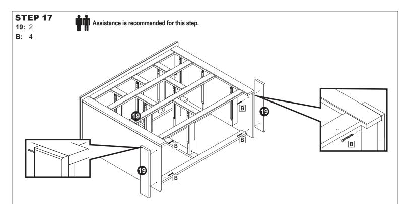
Align two Side Trim Boards (19) with the bottom of the unit, as shown. To ensure the trim boards remain flush with the unit, have an assistant hold them firmly in place while the hardware is secured. From the inside of the side panels, secure each trim board using two M4.5x28mm Pan Screws (B).
