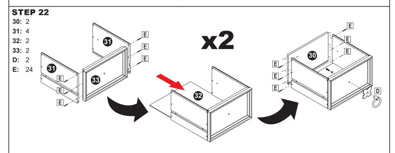
Ensuring the inside grooves align, secure two Large Drawer Sides (31) to Large Drawer Face (33) using six M3.5x30mm Flat Screws (E).
