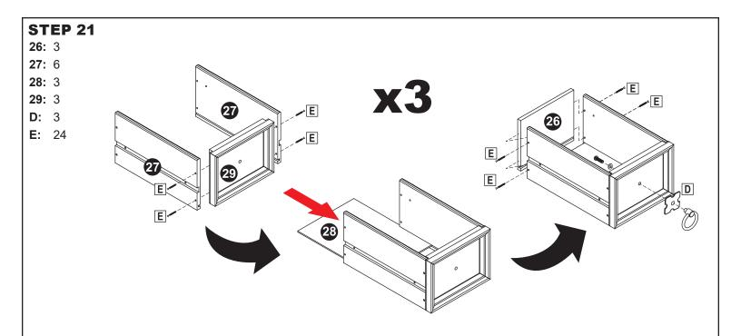
Ensuring the inside grooves align, secure two Medium Drawer Sides (27) to Medium Drawer Face (29) using four M3.5x30mm Flat Screws (E).
