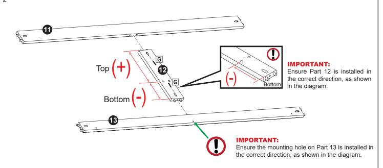
With the angled mounting holes facing upward, lay Bottom Drawer Horizontal Face Frame (11), Bottom Drawer Vertical Face Frame (12), and Bottom Horizontal Frame (13) as shown. **NOTE:** Notice there is a shorter gap between the mounting holes and one end on Part 12, this edge must be installed toward Part 13.
