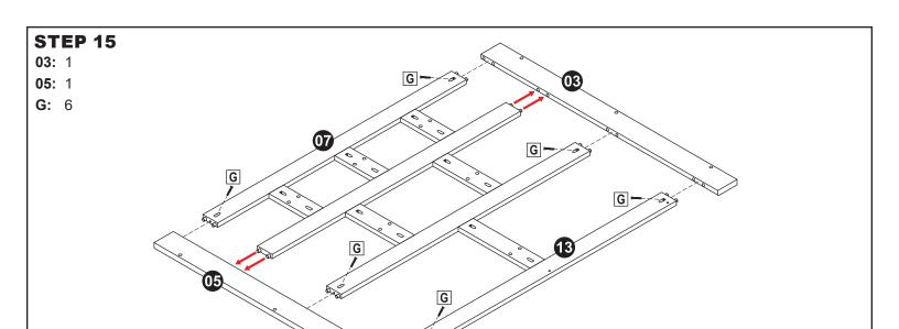
With the dowel mounting holes facing upward, align the Left and Right Stiles (03,05) with the front face frames. Secure each side using three M3.5x25mm Pan Screws (G), as shown.
