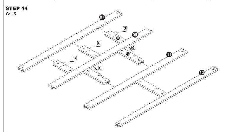
With the angled mounting holes facing upward, align Front Top Horizontal Face Frame (07) with Parts 8. With the angled mounting holes facing upward, align Bottom Drawer Horizontal Face Frame (11) with Parts 10. After components are aligned, secure using M3.5x25mm Pan Screws (G), as shown.
