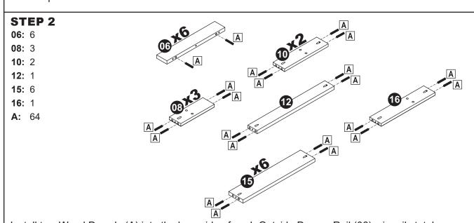
Install two Wood Dowels (A) into the long side of each Outside Drawer Rail (06), six rails total.
