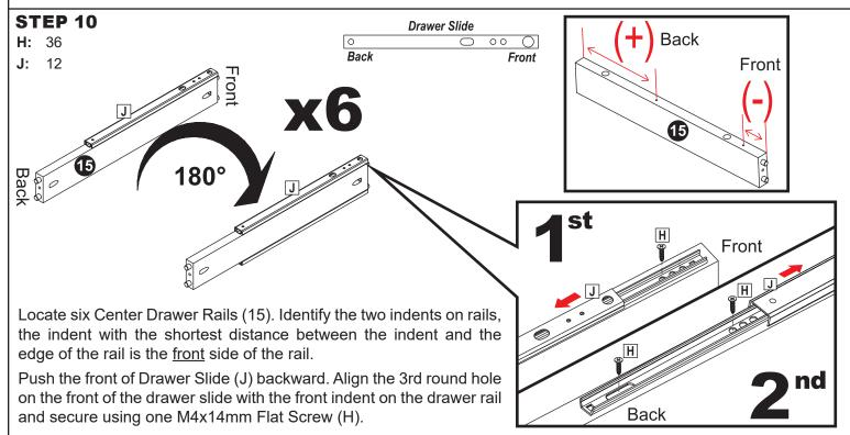
Slide the top piece of the drawer slide forward, the backside indent will align with the 1st small round hole on the back of the slide. Ensuring the slide is centered on the drawer rail, secure the 1st small round hole, then secure the oblong hole using two M4x14mm Flat Screws (H), as shown.
