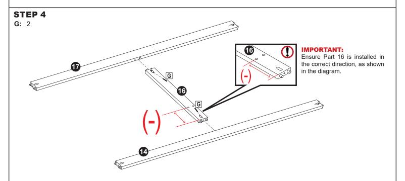
With the angled mounting holes facing upward, lay out Back Bottom Horizontal Support (14), Back Bottom Vertical Support (16), and Back Center Horizontal Support as shown. **NOTE:** Notice there is a shorter space between the mounting holes and one end on Part 16, this edge must be installed toward Part 14.
