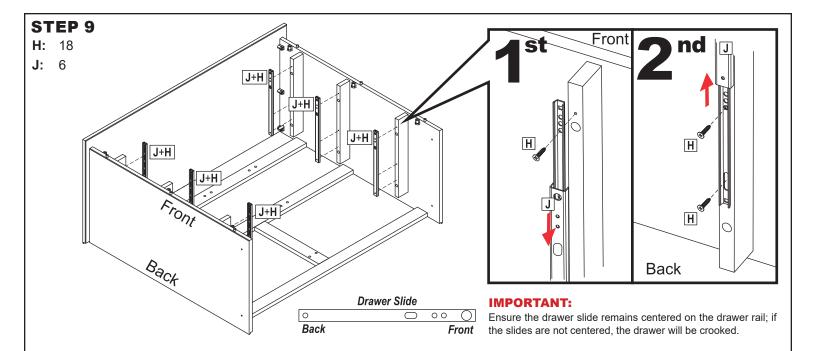
Push the front of Drawer Slide (J) backward. Align the 3rd round hole on the front of the drawer slide with the front indent on the drawer rail and secure using one M4x14mm Flat Screw (H).
