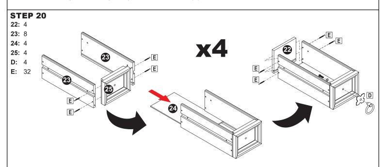
Ensuring the inside grooves align, secure two Small Drawer Sides (23) to Small Drawer Face (25) using four M3.5x30mm Flat Screws (E).
