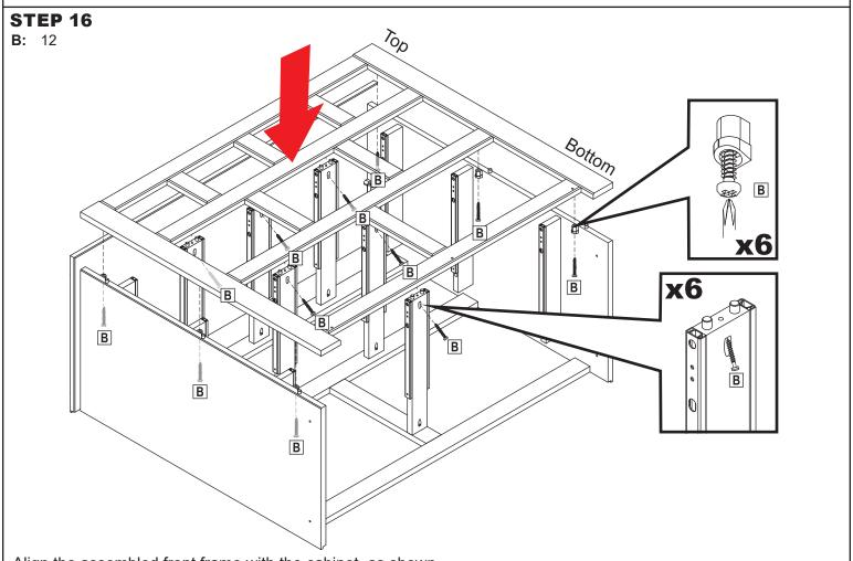
Align the assembled front frame with the cabinet, as shown.
