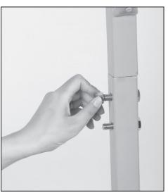
8. Secure the end of the grab bar chain to the holder on the top of the trapeze bar, slide the holder to adjust the position of the triangle grab bar. Fix the holder position by turning the locking pin clockwise.
