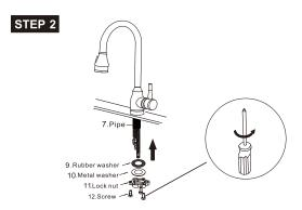
2. Adjust the position of the faucet and secure it with the fixing kit as photo.
