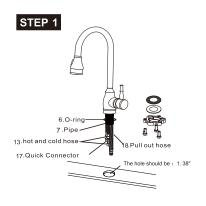
1.Position the faucet,o-ring on the installation surface.And then put the faucet into center hole.
