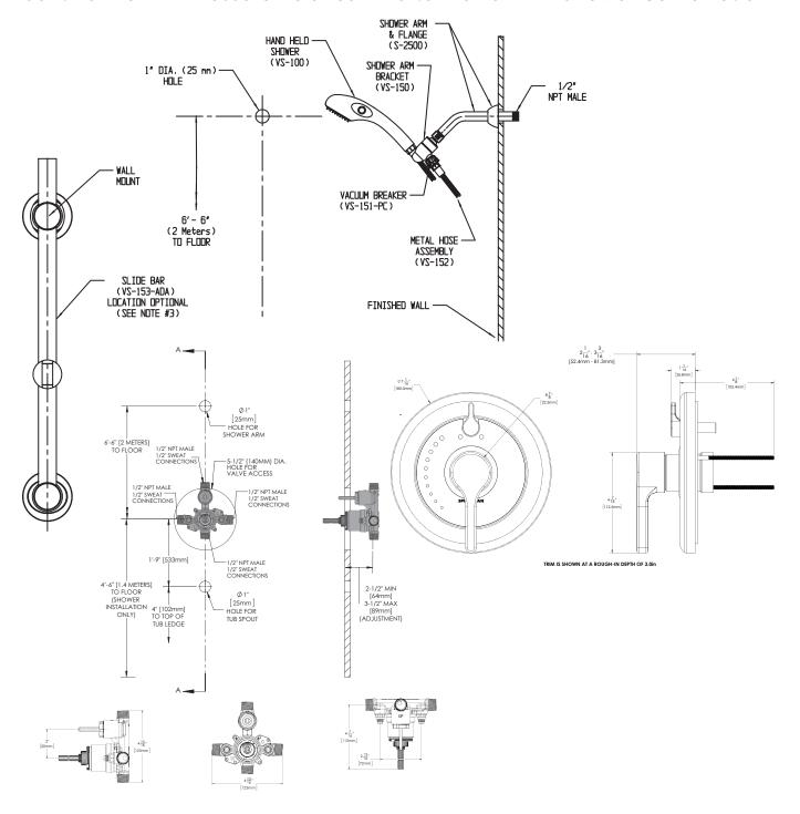
NOTE: 1. All dimensions are in inches (millimeters) unless otherwise specified and are subject to change without notice. 2. Unless otherwise specified, all inlets and outlets are 1/2" female copper sweat. 3. For ADA mounting locations, consult ADAAG, ANSI A117.1, or static regulations
