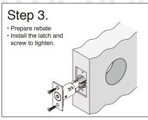
Carefully follow these instructions when installing. Screws to be tightened to a recommended 2.5Nm torque.
