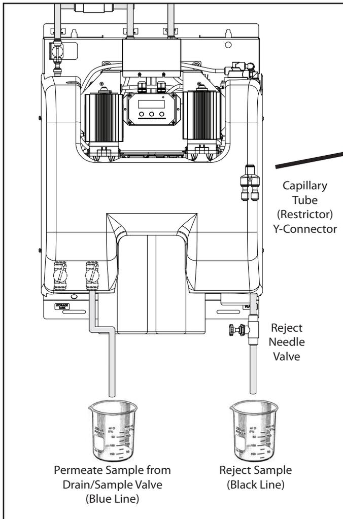
**Figure 6.** Capillary Tube (Restrictor) Y-Connector Detail
