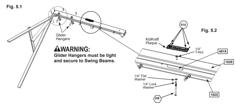
**C:** Attach Swing End Assembly to the side of the Swing Beam Assembly with the overhang (fig. 5.3 & 5.4) using 1 (G5) 5/16 x 4-1/2" Hex Bolt (with lock washer, flat washer and t-nut) in the top hole of Triangle Plate and 1 (G8) 5/16 x 2" Hex Bolt (with 2 flat washers and lock nut) in the bottom hole of Triangle Plate. (fig. 5.3) Make sure Swing End Assembly flares out at an angle. (fig. 5.4)
