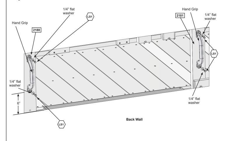
Hardware  $4 \times \sqrt{LS1} \times 1/4 \times 1-1/2$  Lag Screw (1/4" flat washer)
