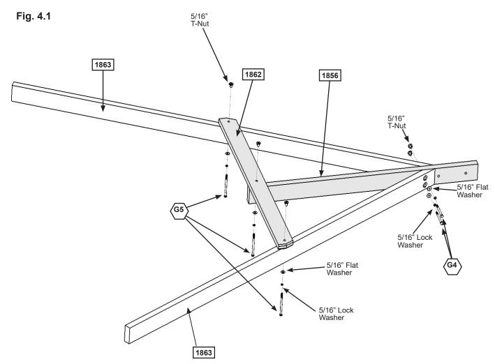
**B:** Attach (1862) SW Support to both (1863) SW Posts and (1856) SW Upright using 3 (G5) 5/16 x 4-1/2" Hex Bolts (with lock washer, flat washer and t-nut). (fig. 4.1)
