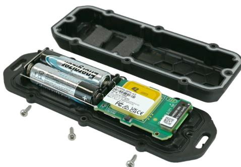
Remove the screws from the tracking device and fit the 2 AA batteries as directed.
