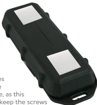
Apply the tape squares to the tracking device as shown in the image, as this positioning is vital to keep the screws accessible for future battery replacement.
