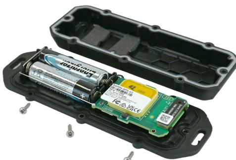
Remove the screws from the tracking device and fit the 2 AA batteries as directed.
