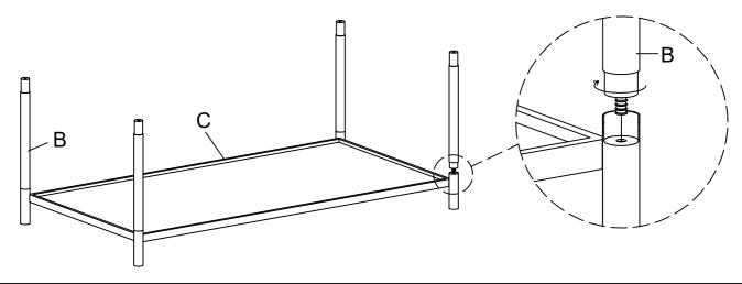
Assemble the Shelf Panel (D) with Post (B) step by step from the bottom to top as below shown.
