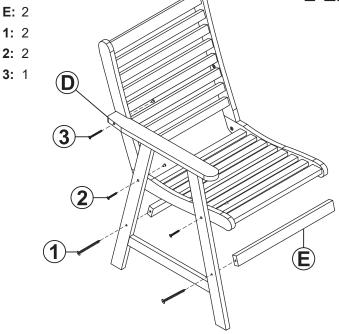
Secure Right Arm Panel (D) to the seat using two M6x30mm Bolts + Cap (2).
