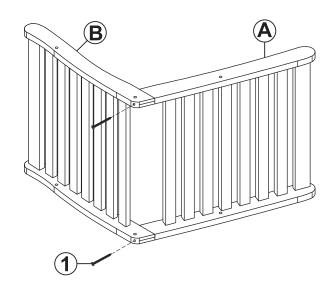
Secure Seat (B) to Backrest (A) using two M6x60mm Screws (1).
