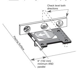
**Step 6:** Position 5" ground anchor (Item G2550) in center of hole with hinge side toward and parallel with playing surface. Using a level, ensure the anchor is level front-to-back and left-to-right. All edges of the ground anchor must be 6" (15.2 cm) away from all sides of hole and the top of the ground anchor within a range of 1"- 3" (25-75 mm) above the level of the playing surface.
