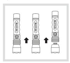
NOTE: Turn the light off prior to removing the head. If the light is not turned off, the base will remain on.
