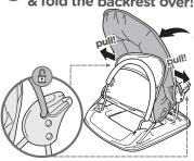
Release support legs from bather base by rotating the legs until key can slide out of slot!
