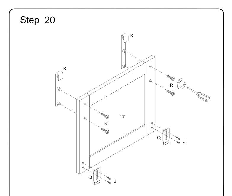
Using bolt (R) secure pulley (K) into part (17) ,then using screw (J) attach plate (Q) into part (17) with Philips head screwdriver as per diagram.
