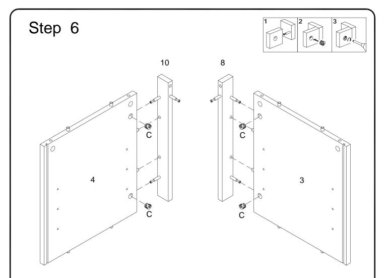
Using cam lock(C) secure part (10) into part (4) ,part (8) into part (3) with Philips head screwdriver as per diagram.
