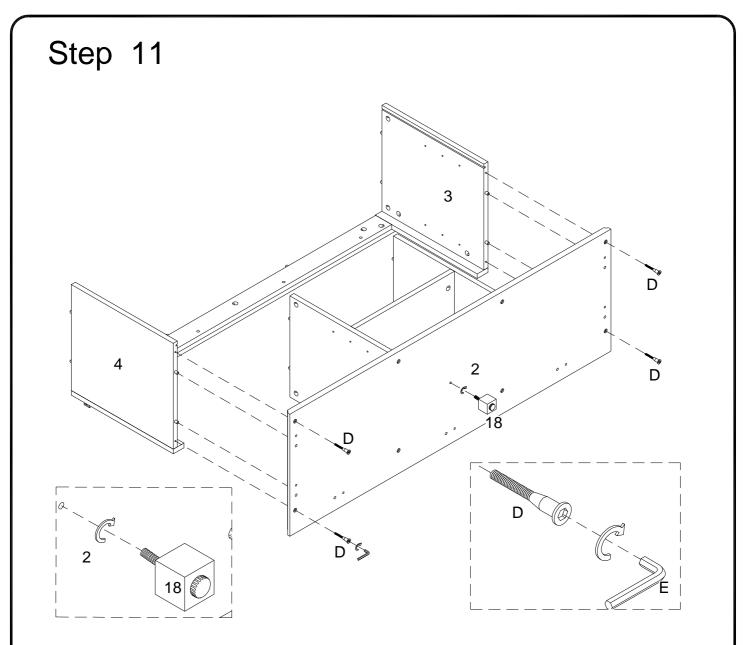
Secure part (18) into part (2),then using screw (D) attach part (2) into parts (3,4) with hex key (E) as per diagram.
