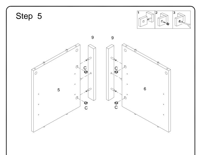
Using cam lock(C) secure part (9) into parts (5,6) with Philips head screwdriver as per diagram.
