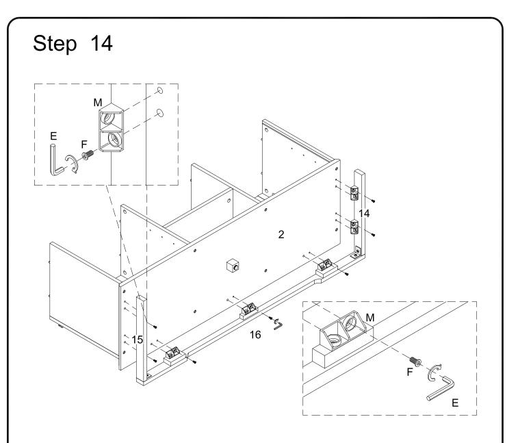
Using bolt (F) attach connector (M) to part (2) with hex key (E) as per diagram.
