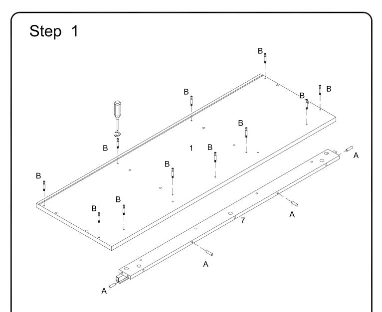
Insert wooden dowel (A) into part (7), then secure cam bolt (B) into part (1) with Philips head screwdriver as per diagram.
