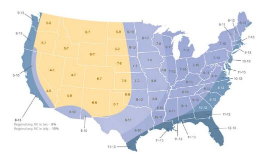
Note: Actual moisture content conditions in any location may differ significantly from these numbers. This map cannot be reliably used as a basis for installation. The most reliable moisture-content numbers can be obtained at the job site.
