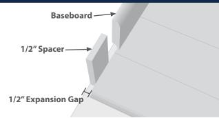
Leave at least 1/2" expansion spaces between flooring and ALL vertical objects (walls, cabinets, pipes, etc.) Large flooring runs may require additional expansion space. For floating floors, use transition moldings between rooms and doorways 3ft. or less. Undercut door jambs and casings to provide adequate expansion space. Do not screw or nail cabinetry or other permanent fixtures to a floating floor.
