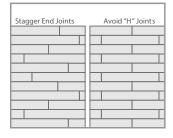
Note: Although H joints do not void a warranty, they can decrease the overall structural strength of the flooring therefore Cali never recommends H joint installation.
