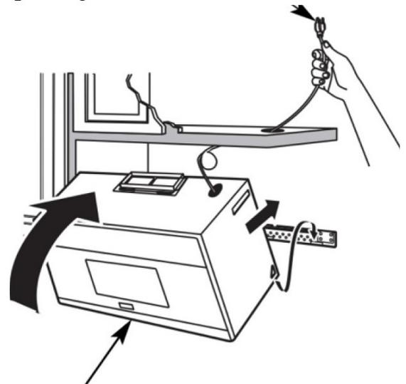
Bertazzoni recommends to operate the appliance after it has been installed in a cabinet. The kitchen cabinets shall be made of materials capable of withstanding temperatures at least 117°F (65°C) above room temperature in order to avoid possible damage to the cabinets during oven usage.
