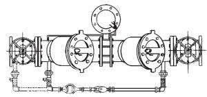
**NOTE:** Piping for 3" 909 will start from #1 gate valve and connect at #2 check valve.
