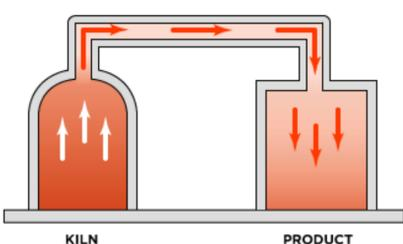
Waste heat from the kilns is routed to the product dryer. This reduces 15% natural gas consumption.
