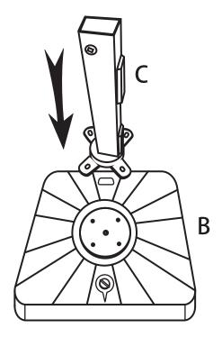
**Step 3** Fix the Base Pole (part C) on the top of the Plastic Water Fillable Stand (part B) with bolts F & washers G use the Allen Wrench (E)
