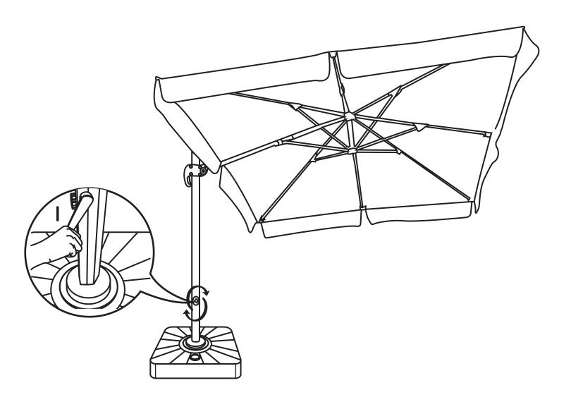
**Step 12** Squeezing the trigger before attempting to lower the crank house. Turn the Crank handle counter-clockwise to close the umbrella.
