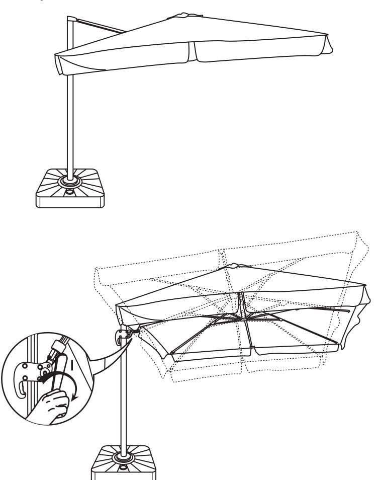
**Step 11** Fix the Crank Handle (I) into the bottom crank hole to rotate your umbrella in 360 degrees.
