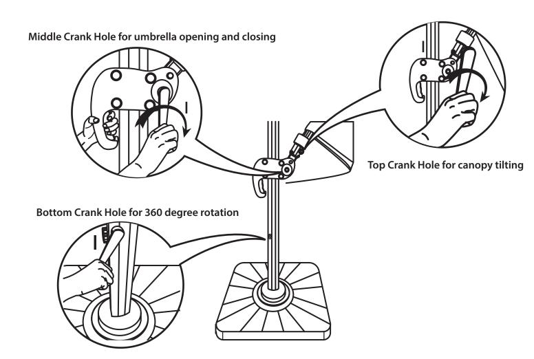
Step 8 Squeezing the trigger before attempting to raise the crank house. Fix the Crank Handle (I) into the middle crank hole and turn clockwise to extend the umbrella fully.
