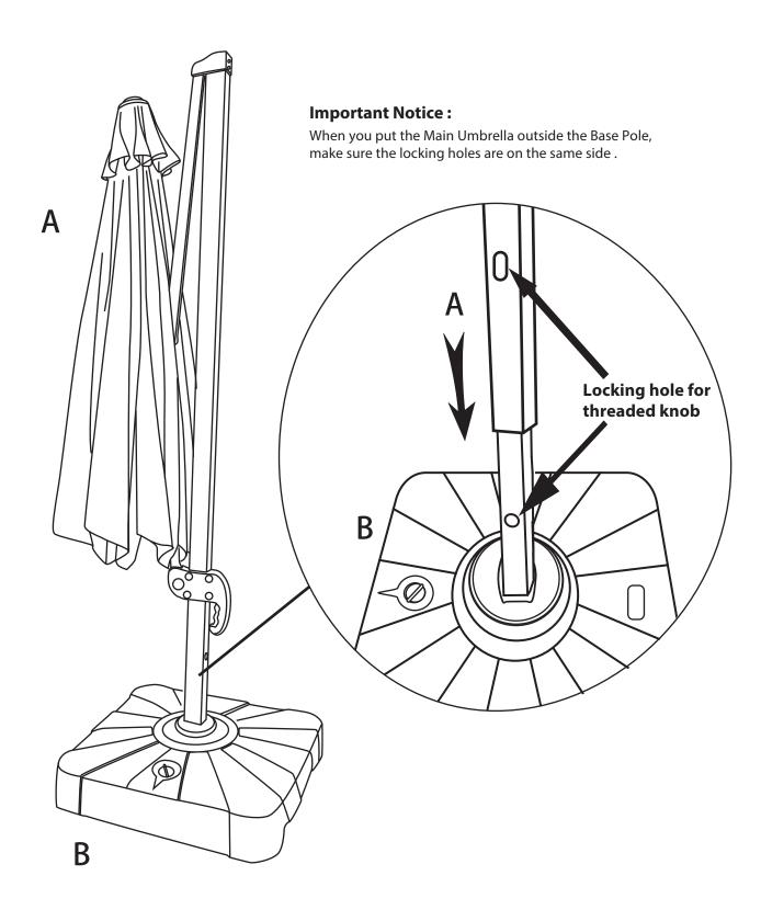
**Step 6** Fix the Threaded Knob ( Part H ) into the locking hole.
