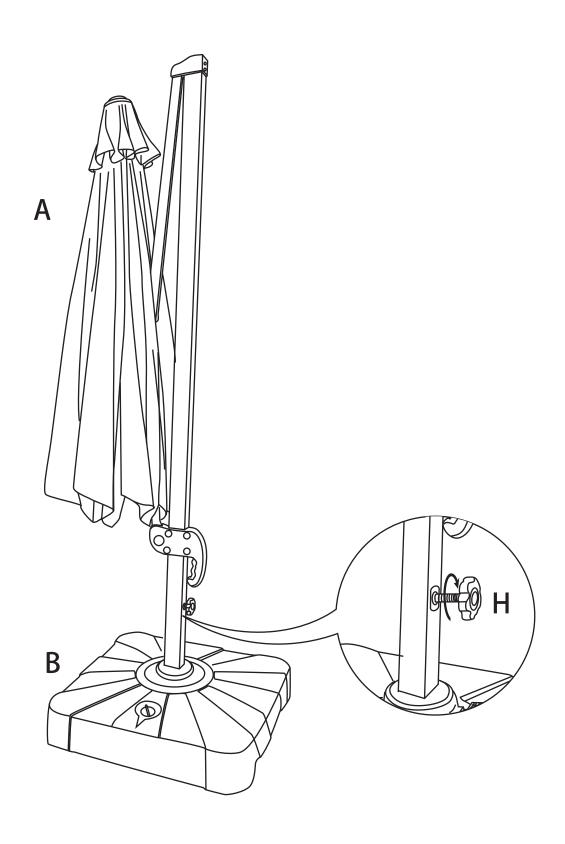
**Step 7** There are 3 Crank Holes on your umbrella. Top crank hole for canopy tilting, Bottom crank hole for 360 degree rotation. Middle crank hole for umbrella opening and closing.
