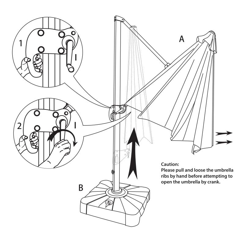
**Step 9** The umbrella has 6 position holes on the main pole to fix the canopy at different angles .
