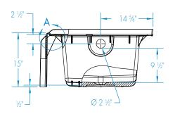
FEATURES Dimensional Tolerance ± 3/8". Dimensions needed for site preparation should be measured from the unit. Manufacturer assumes no responsibility for preparatory work.
