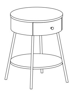
This page lists all the contents included in the box. Please take the time to identify the hardware as well as the individual components to this product. As you unpack and prepare for assembly, place the contents on a carpeted or padded area to protect them from damage. Attach Leg (C) to the Shelf (B) using Bolt (D), Lock Washer (F), Flat Washer (E), on holes of Leg (B). Turn the Allen Key (G) in Bolt (D).
