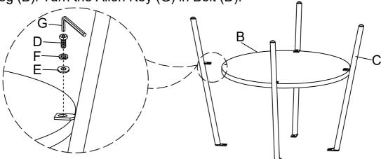
Attach Leg (C) to Table Top (A) using Bolt (D), Lock Washer (F), Flat Washer (E), on holes of Leg (C). Turn the Allen Key (G) in Bolt (D).
