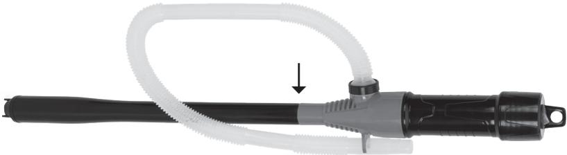
If pumping flammable liquids, fuels, heating oils: The pickup tube/pump body connection must be inside the container the fuel is coming from as the pump is designed to seep at that joint.
