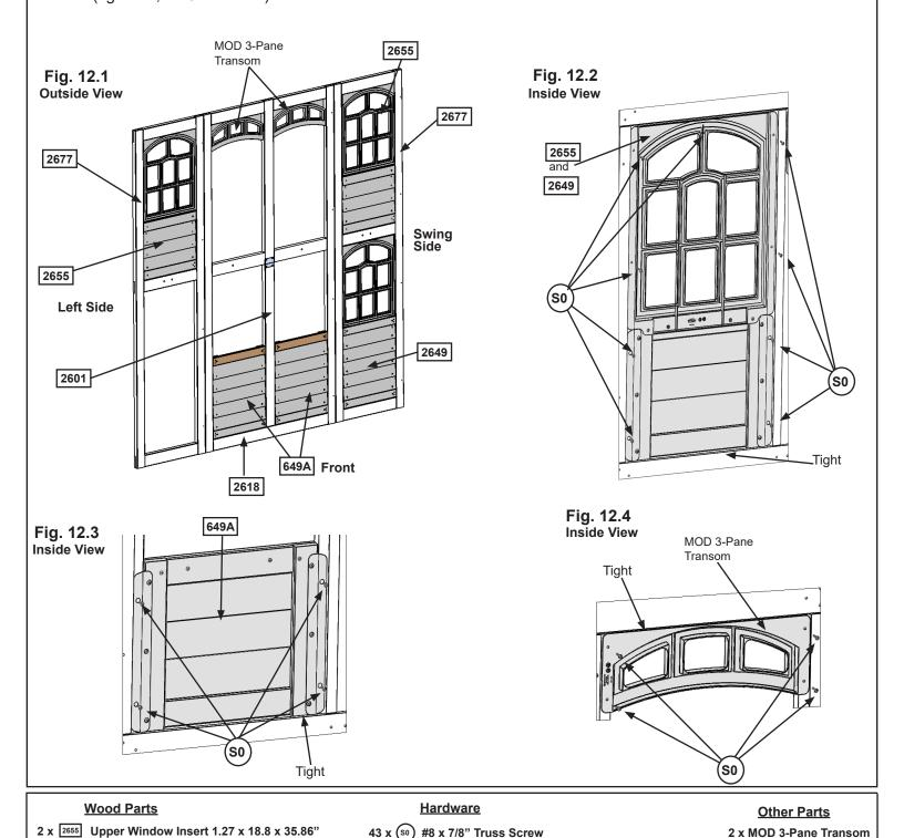
1 x 2649 Lower Window Insert 1.27 x 18.8 x 41.91" 2 x 649A Short Half Wall 1.27 x 18.8 x 20-15/16"
