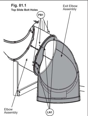
After the clamp rings are attached to the elbows, fasten them end to end with two pan bolts and lock nuts
