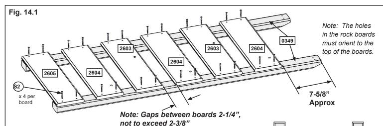
A: Lay 2 (0349) Rock Rails down, side by side with angled edges facing down. (fig. 14.1)
