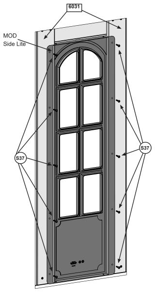
Note: Do NOT use top/bottom screw hole to attach window, sides only.
