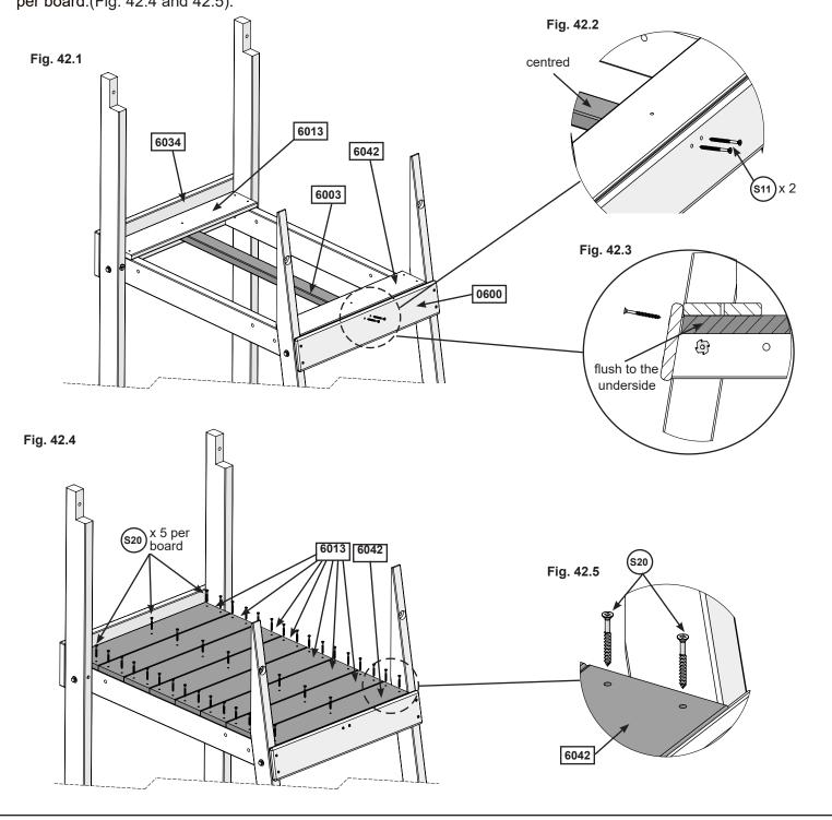
1 x 6003 Floor Joist 15/16 x 2 x 33-15/16" 6 x 6013 Floor Board 5/8 x 4-1/4 x 21"
