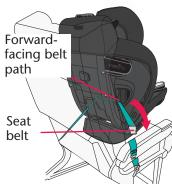
Adjust the child restraint to **Recline Position #5** (p. 58), then place it on the aircraft seat forward-facing.
