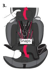
Unfasten two snaps at the harness slot openings where the shoulder straps come out then unfasten snaps on the inside of the seating area.
