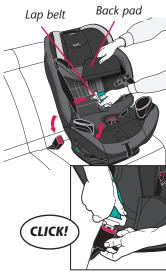
Raise headrest to its highest position (p. 58), then lift back pad away from child restraint for easier access. Route the lap belt through the forward-facing belt path and continue through the opposite opening of the child restraint. Fasten the buckle.
