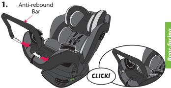
Place Anti-rebound Bar through slots in seat cover into metal tubing in seat shell.
