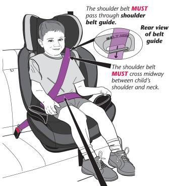
The lap belt is stretched low and snug across the child's hips, within the lower belt guides, and fastened into the buckle.
