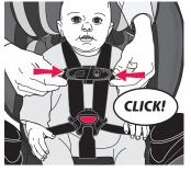
Snap the two halves of the chest clip together, as shown, and slide to armpit level.
