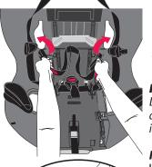
**IMPORTANT:** Make sure the Lower Anchor Connector strap does not interfere with the internal harness straps.
