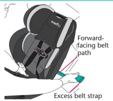
The aircraft seat belt must be as tight as possible. Route the excess aircraft seat belt strap back through the forward-facing belt path opening, as shown. Using your full weight, push the child restraint firmly onto the aircraft seat while pulling on the excess seat belt strap to tighten.
