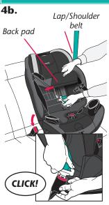
Raise headrest to its highest position (p. 58), then lift back pad away from child restraint for easier access. Route the lap/shoulder belt through the forward-facing belt path and continue through the opposite opening of the child restraint. Fasten the buckle.
