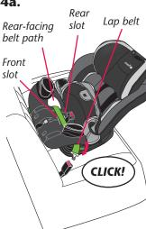
Pull the seat pad off of the front of the child restraint. Route the lap belt through the rear-facing belt path and continue through the opposite opening of the child restraint. Fasten the buckle.
