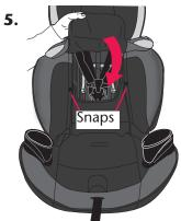
Raise back pad and fasten the two snaps on side of seat pad then lower the headrest pad.
