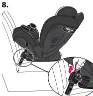
To remove the lower anchor connector assembly strap, pull red release strap. Remove the other strap on the other side of the seat from the vehicle anchor.
