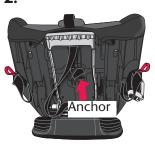
Remove the crotch buckle from the crotch slot.
