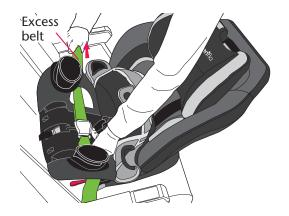
The aircraft seat belt must be as tight as possible. Route the excess seat belt strap back through the rear-facing belt path opening, as shown above. Using your full weight, push the child restraint firmly onto the aircraft seat while pulling on the excess seat belt strap to tighten.
