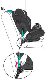
To remove the lower anchor connector assembly strap, pull red release strap. Remove the other strap on the other side of the seat from the vehicle anchor.
