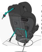
Tighten the strap by moving the handle back and forth on the lower anchor connector as shown until the seat is tight. Fold handle up after tightening.
