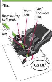
Pull the seat pad off of the front of the child restraint. Route the lap/shoulder belt through the rear-facing belt path and continue through the opposite opening of the child restraint. Fasten the buckle.
