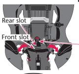
IMPORTANT: If crotch buckle is in rear slot, place lower -anchor (UAS) strap in front of buckle. If crotch buckle in front slot, place lower anchor (UAS) strap behind buckle.
