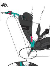
Attach lower anchor / UAS connectors to the vehicle lower anchor bars until they lock onto the bars on both sides of the seat.
