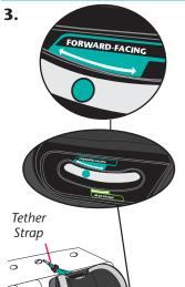
Place child restraint in your vehicle forward-facing, as shown. Always make sure the bottom of the child restraint sits flat on the vehicle seat.
