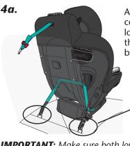
Attach lower anchor (UAS) connectors to the vehicle lower anchor bars until they lock onto the bars on both sides of the seat.
