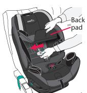
Route the aircraft seat belt through the forward-facing belt path opening in the back of the child restraint and continue through the belt path opening on the opposite side of the child restraint.
