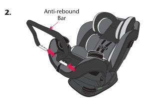
To remove the Anti-rebound Bar, press both locking buttons and withdraw the Bar from the seat
