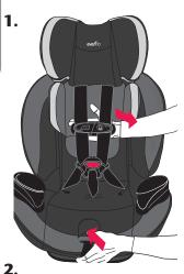
Loosen harness straps by pushing the harness release button on the front of the seat. At the same time, pull on the harness straps.
