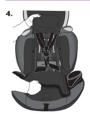
Reassemble the loose crotch buckle onto the shoulder straps and fasten the chest clip.
