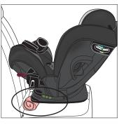
**Note:** In some vehicles, in **Position 1**, it may be necessary to place a tightly rolled towel or small blanket beneath the front edge of the child restraint to provide enough recline so that the leveling ball is in the green zone for rear-facing use.
