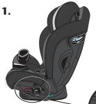
Re-route the lower anchor connector strap through the rear-facing belt path (p. 28). Store the lower anchor connector (UAS) in the rear-facing belt path as shown.
