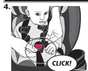
Insert both buckle tongues into the buckle. Pull up on the harness strap to check that the buckle tongues are fastened and to remove any slack from the webbing around the child's legs.
