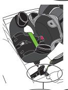
Tighten the strap by moving the handle back and forth on the lower anchor connector as shown until the seat is tight. Fold handle up after tightening.
