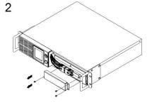
Remove the three retaining screws of the cable protection cover then remove the cover.
