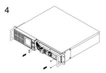
Remove the four retaining screws.
