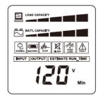
The LCD display indicates a variety of UPS operational conditions. All descriptions apply when the UPS is plugged into an AC outlet and turned on or when the UPS is on battery.
