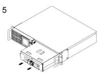
Insert the new battery pack. Assemble the screws, cover, cable and front panel in the reverse sequence of above steps. Recharge the unit for 4-8 hours to ensure the UPS performs expected runtime.
