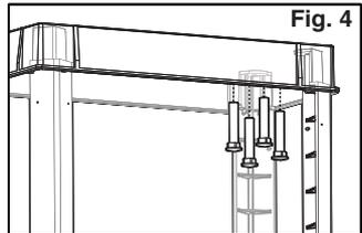
**NOTE:** To maximize control, we suggest installing the fixed casters on the same side as the handle, while the swivel casters go on the opposite side of the cart. However, if you prefer to have them the opposite way in order to make sharper turns and pivots, that will also work.
