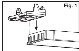
**NOTE:** To overcome the friction between the two plastic surfaces, rub a little petroleum jelly onto the grooved surface. The two parts should slide together with a few gentle taps of the rubber mallet.
