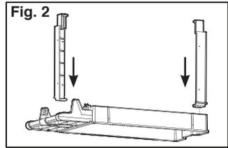
4. Insert and tighten three screws per leg so that the legs are secured in the shelf tray.
