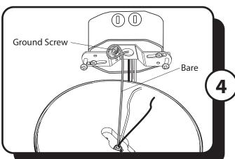
4. Loosen the ground screw on the mounting bracket and wrap the bare wire from the fixture around the ground screw. Tighten the ground screw to hold the bare wire in place. **Note:** Ensure there is enough of the bare wire extending from the ground screw to connect to the ground wire from the outlet box using a wire connector.
