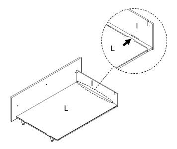
Insert another Drawer Side Board (I) to the Drawer Bottom Board (L) first, and attach the Drawer Side Board (I) to the Drawer Bottom Frame (K), then insert the Bolt (X) and Washer (AD), turn the Ratchet Tool (AF) to tighten them.
