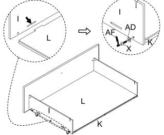
122 Attach the Drawer Back Board (J) to the Drawer Bottom Frame (K), insert the Bolt (X) and Washer (AD), turn the Ratchet Tool (AF) to tighten them. Attach the Drawer Board Connector (Q) to the assembled drawer, insert them into correct places.
