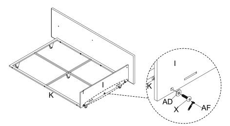
Insert the Drawer Bottom Board (L) to the assembled Drawer Side Board (I).
