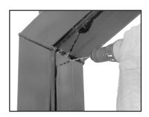
**Step 5:** On the back side of pole, drill another 11/64" hole – centered on pole and 3/16" down from the weld.
