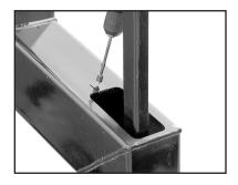
**Step 4:** Using a 5/16" hex head driver, install a #10 – 16 x 3/4" screw into hole that was just drilled.
