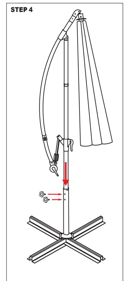
Firmly insert the Umbrella into the assembled base. Screw in and tighten the Threaded Knobs into the pole support.
