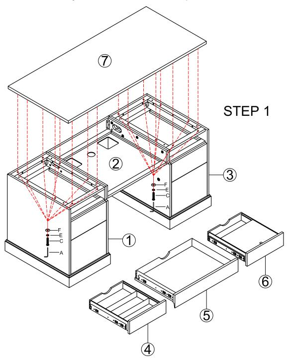
Step 1: Take out all drawers (4, 5 & 6), then loosen bolts (C), lock washers (E) and flat washers (F) by using allen wrench (A) and remove top panel (7) from the desk.
