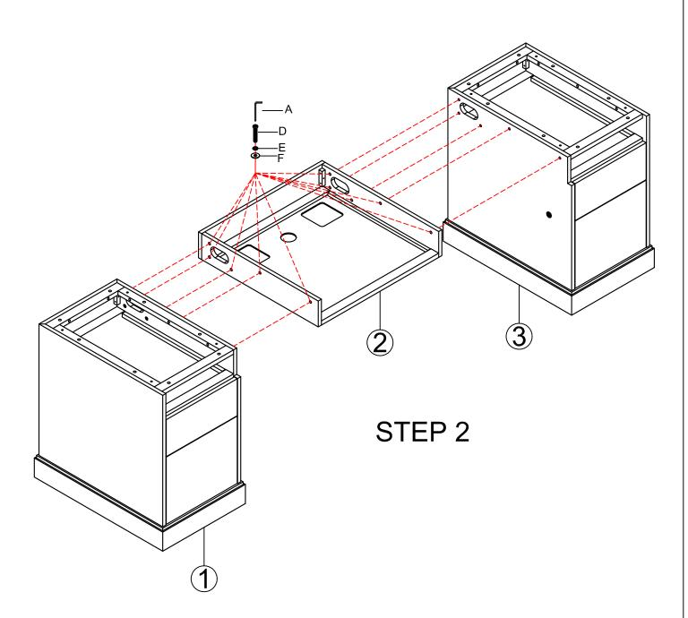
Step 2: Loosen bolts (D), lock washers (E) and flat washers (F) with allen wrench (A), then remove center frame (2) from the left and right pedestals (1 & 3).
