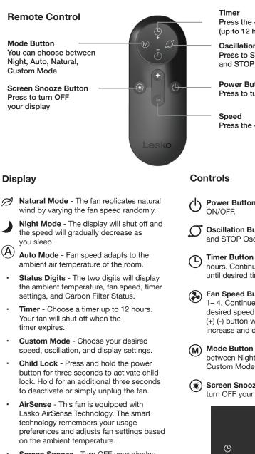
Screen Snooze - Turn OFF your display for easier night time use. When display is in Snooze Mode, indicators will light up temporarily anytime a button is pressed then shut off.
