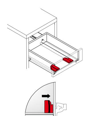
Unlatching the drawer and removing it from the runners is just as easy.
