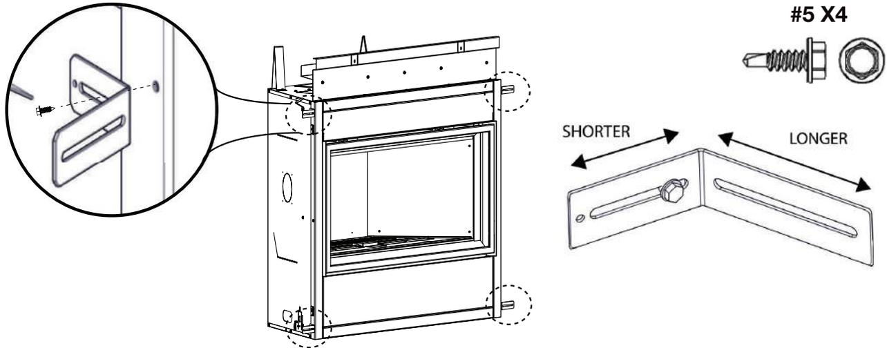
Use one screw to secure the short side of the nailing bracket to the appliance. Repeat for 3 other locations.
