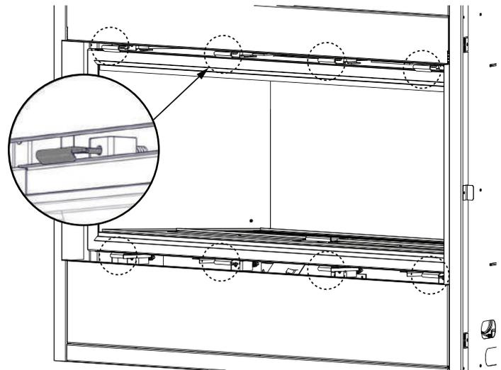
Leave a hand on the glass door during entire door removal. The glass door is secured to the firebox with four (CBLX42), six (CBLX46), or eight (CBLX56) spring latches. Pull the handles of the latches forward, then lift/lower the latches out from the door frame to release the door. Next, lift the door up until the bottom edge clears the bottom shoulder screws of the appliance. Carefully grip the top and bottom of the door lifting it off the appliance.
