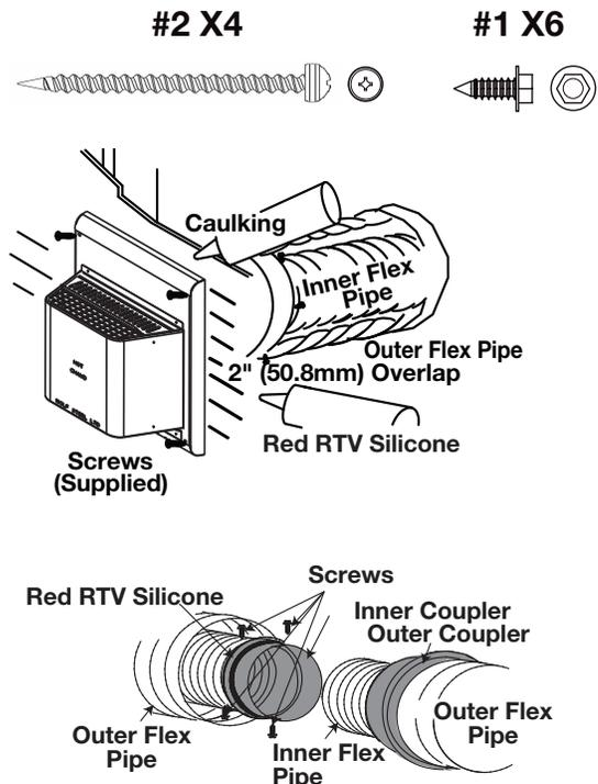
**The air terminal mounting plate may be recessed into the exterior wall or siding no greater than the depth of its return flange.**
