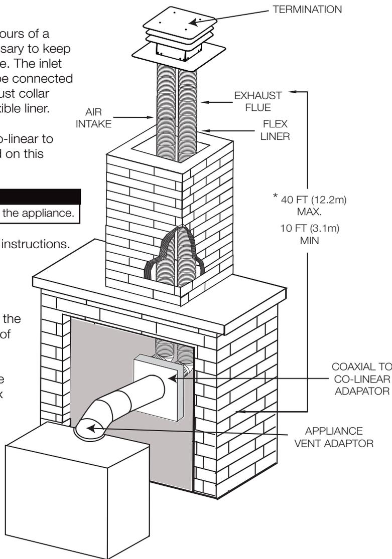
\* Measured from appliance flue collar to termination flue collar
