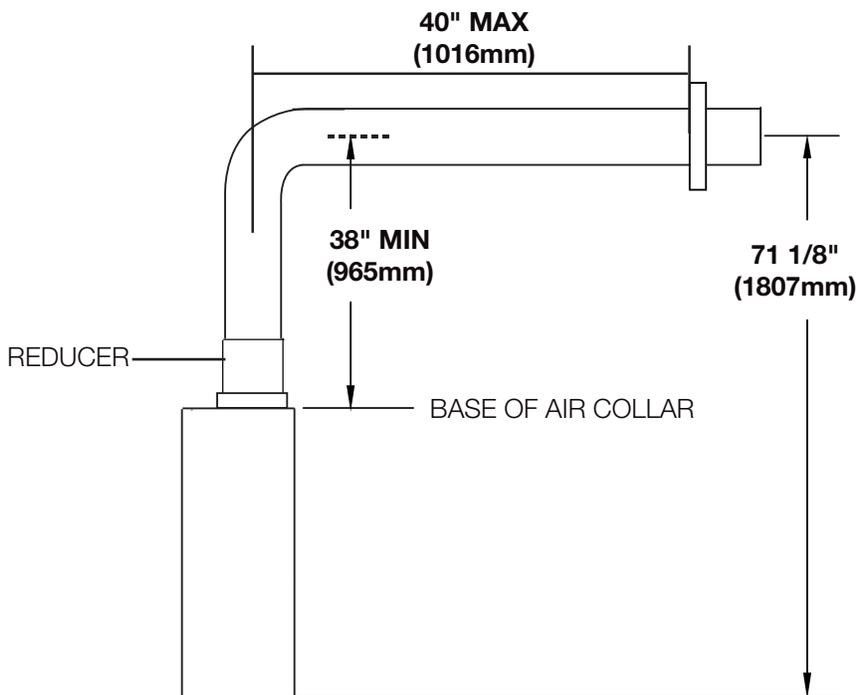
**For 4" / 7" (Use reducer kit A4758AK to transition from 5" / 8" to 4" / 7" venting)**
