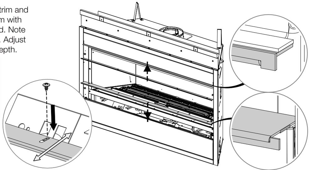
3. Install the left (L) and right (R) trims with the flanges facing outward. Adjust the trims to the desired depth and tighten the screws and shoulder bolts.
