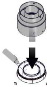
USE MILL PAC TO SEAL REDUCER TO THE APPLIANCE EXHAUST COLLARS.
