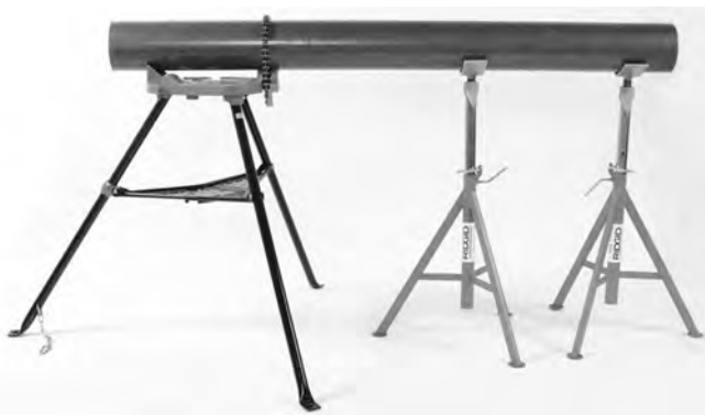
Figure 7 – Example of Pipe Support
