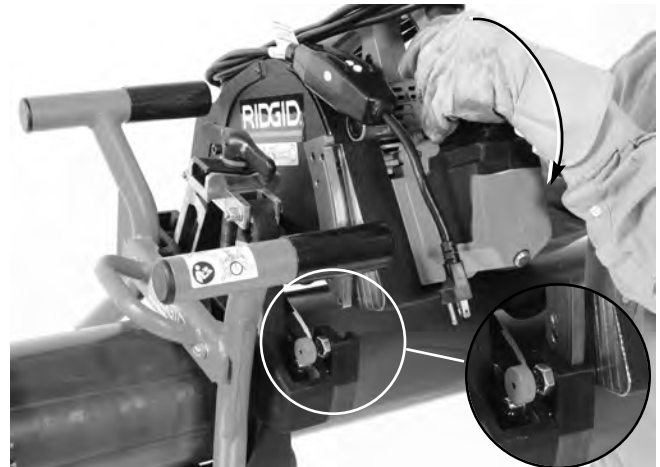
Figure 12 – Engaging Plunge Plate Into Guide
