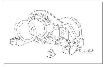
5. Place the four fiber washers onto the capstan shaft. Install the new capstan unit (5) so that the antirotation support unit engages the hole in the antirotation plate. Install the capstan bolt.
