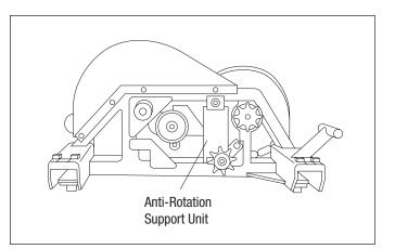
4. Install the anti-rotation support unit (4) as shown and slide rearward, so the bottom of the support unit is trapped behind the idler sprocket mounting plate.
