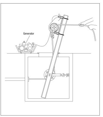
Using a Manhole Sheave
