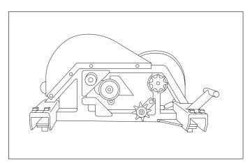
3. Slide the capstan unit off of the capstan shaft. Remove four fiber washers.
