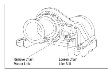
2. Loosen the chain idler arm bolt. Slide the idler down to loosen the chain. Remove the chain master link. Remove the chain.
