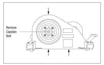
1. Remove the chain guard screws as shown. Remove the chain guard. Remove the capstan bolt.
