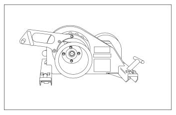
9. Attach the new capstan arm (1) to the ramp (13) with the three cap screws (2) and washers (3).
