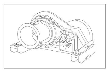
7. Slide the idler arm up until the chain is snug. Tighten the idler arm bolt.
