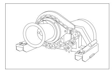
6. Feed the chain onto the bottom side of the sprocket while turning the sprocket clockwise. Install the new connecting link (5). So that the open end of the connecting link faces away from the direction of the chain travel.
