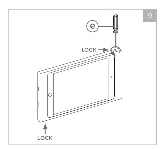
To lock the Surface Mount in place, use the (e) security tool provided to engage the security locks. When the bezel is in landscape orientation, the security holes are located on the top-right and bottom-left of the bezel. Rotate the (e) security tool counter-clockwise to engage the locks, and clockwise to unlock the Surface Mount (a) bezel from the (b) mounting bracket.
