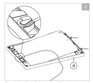
Plug in the iPad's lightning to USB cable directly into the iPad. Position the iPad facedown into the (a) bezel with the iPad cable on the left. Carefully wrap the iPad cable around the metal loop located on the (a) bezel. To lock the iPad in place, use a flat head screwdriver to deploy the second and third toggles located on the right side of the Surface Mount (a) bezel. The first top-right toggle is a power button extension. Note: iPad Pro 12.9" Bezel contains three toggles.
