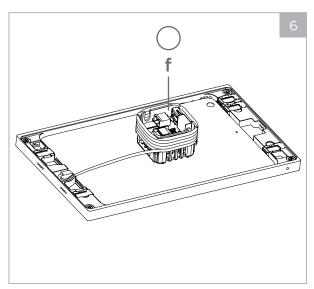
Connect the USB connector to the USB port located on the (f) PoE splitter. Tightly wrap the remaining iPad cable around the (f) PoE splitter. Leave enough slack on the iPad cable to place (f) PoE splitter into the electrical box.
