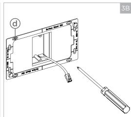
Using the recommended screwdriver and (d) mounting screws, install the first screw in the upper left-hand corner.
