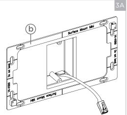
Install the (b) mounting bracket on the wall with the (b) bracket surrounding the electrical box. Use the center lines as a guide to install the (d) mounting screws. Our specialized (d) mounting screws act as anchors and screws when mounting on a drywall or wood surface.
