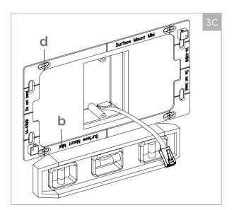
Level the (b) mounting bracket over wiring location and fasten (b) bracket with the remaining (d) screws. Lining up the (d) mounting screws with the engraved center lines provided on the (b) bracket will allow you optimal adjustability. The (b) mounting bracket is now in
