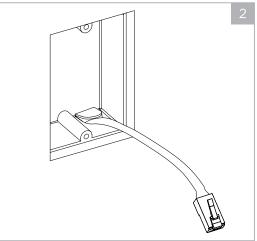
Locate the ideal mounting area. For retrofit installation. locate an existing low-voltage electrical box. For new construction, choose a location for an electrical box. We recommend installing the (a) bezel in landscape orientation, but it can also be installed in portrait orientation. **Note:** A single gang electrical box allows
