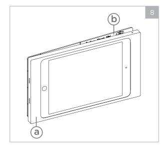
With the iPad home button facing left or right, the Surface Mount will attach to the (b) mounting bracket with internal magnets.
