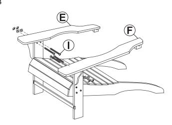
Loosely fasten Right Armrest (E) to the right leg using two Bolt Sets (I).
