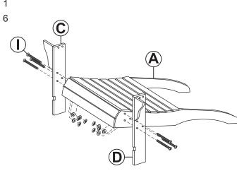
Attach Right Leg (C) to Seat (A) by hand-tightening three Bolt Sets (I).
