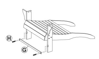
Secure Leg Support (G) to the front of the legs using four Screws (H).
