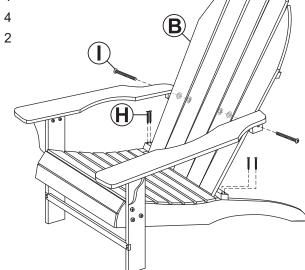
Secure Seat (B) to the back of the armrests using two Bolt Sets (I).
