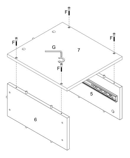
Using screw (F) attach part (7) to parts (5,6) with hex key (G) as per diagram.
