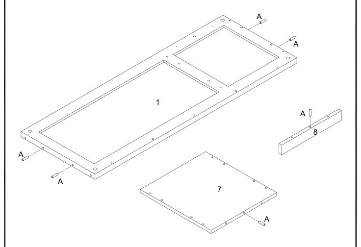
Insert wooden dowel (A) into parts (1,7,8) as per diagram.
