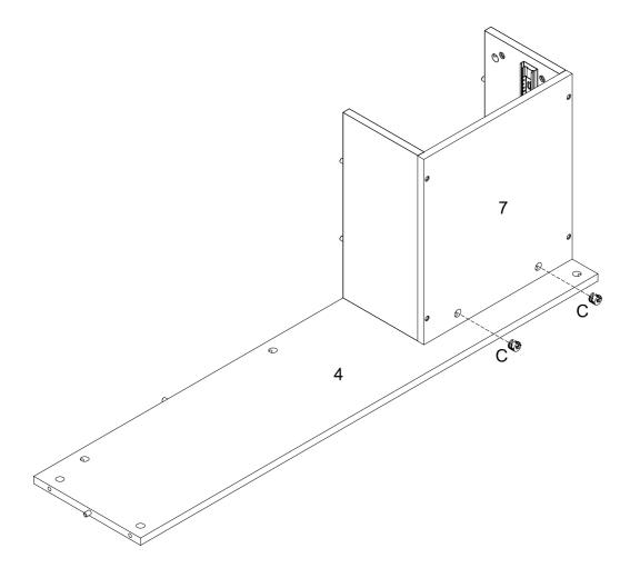
Using cam lock(C) secure part (7) to part (4) with Philips head screwdriver as per diagram.
