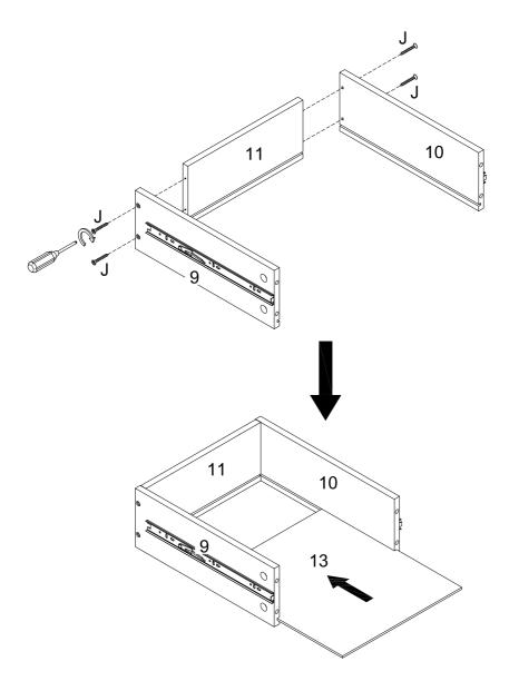
Using screw (J) attach parts (9,10) to part (11) with Philips head screwdriver as per diagram. then put part (13) as per diagram.
