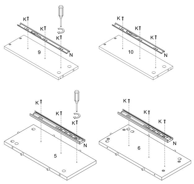
Using screw (K) attach slider (N) to parts (5,6,9,10) with Philips head screwdriver as per diagram.
