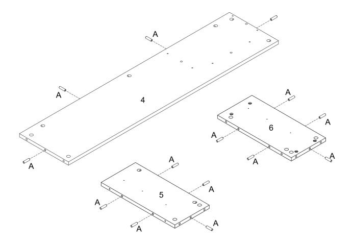
Insert wooden dowel (A) into parts (4,5,6) as per diagram.
