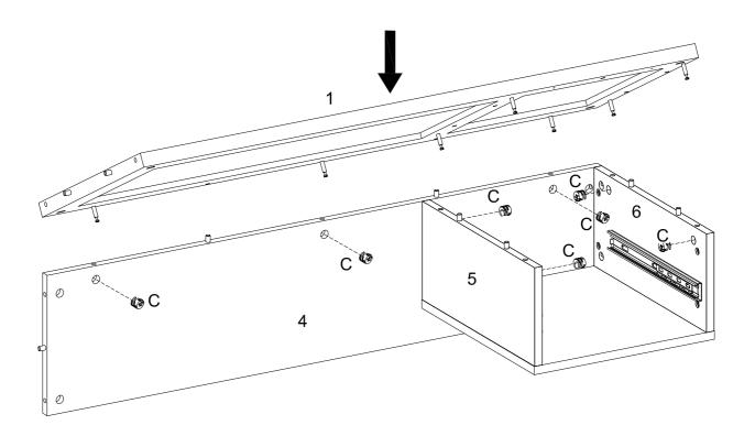
Using cam lock(C) secure part (1) to parts (4,5,6) with Philips head screwdriver as per diagram.
