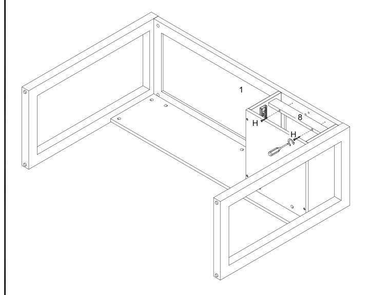
Using screw (H) attach part (8) to part (1) with Philips head screwdriver as per diagram.
