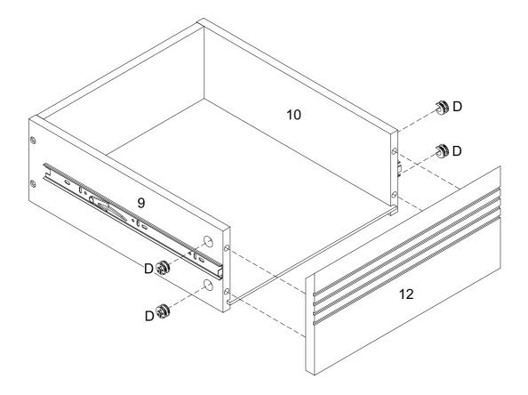
Using cam lock(D) secure part (12) to parts (9,10) with Philips head screwdriver as per diagram.
