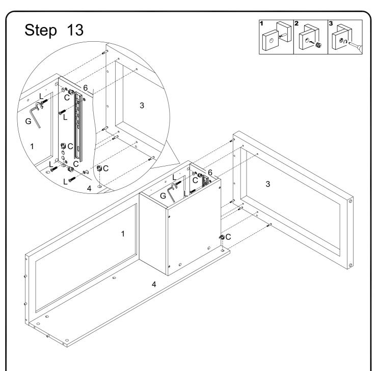
Using cam lock(C) secure part (3) to parts (1,4) with Philips head screwdriver, then using bolt (L) attach part (6) to part (3) with Hex key (G) as per diagram.
