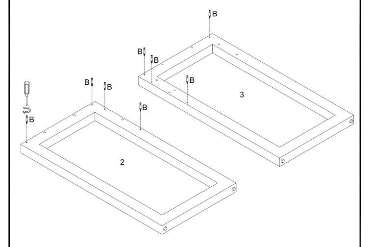
Secure cam bolt (B) into parts (2,3) with Philips head screwdriver as per diagram.
