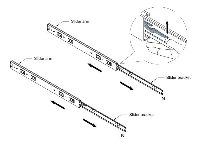
Pick up the slider arm (N) and separate the slide Runner for the following Steps. Extend the Slide .Runner all the way forward,press the plastic release lever of the slider arm up and pull the Slide Runner Complete out .
