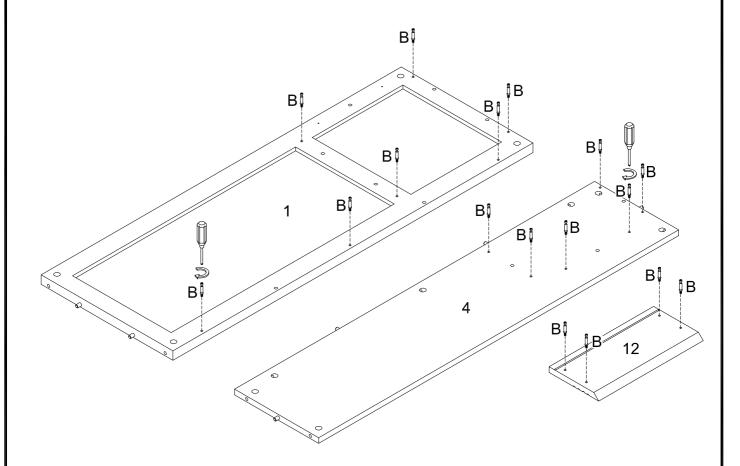
Secure cam bolt (B) into parts (1,4,12) with Philips head screwdriver as per diagram.
