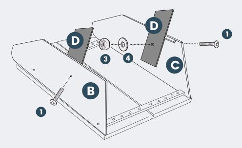
**4** Tighten all the screws when the parts are loosely attached.
