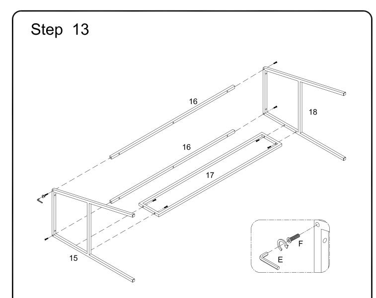
Using bolt (F) attach parts (15,18) to parts (16,17) with hex key (E) as per diagram. Note : Do not fully tighten all the bolts .
