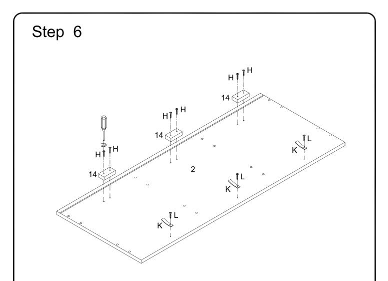
Using screw (H) attach part (14), screw (L) attach plastic wedge (K) to part (2) with Philips head screwdriver as per diagram.
