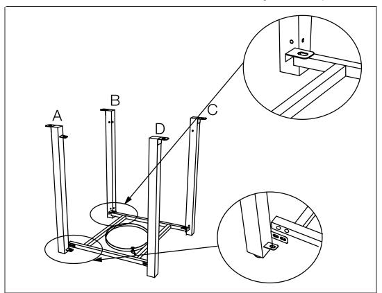
1. Connect the tank holder/base (I) With table Lets(A/B/C/D) by 6pcs screws (O).
