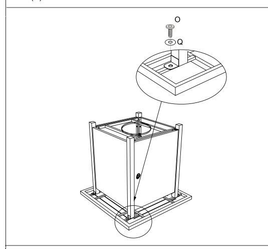
4.Attach the assembled base to the bottom of top using 4pcs of screws (O), and 4pcs M6 washers(Q), make sure the panel (L) faces the valve stem. Tighten all screws.
