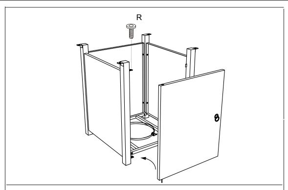
3. Hang the bottom (H) of the door plate on the round bracket. Top with 1PC screw(R)lock.
