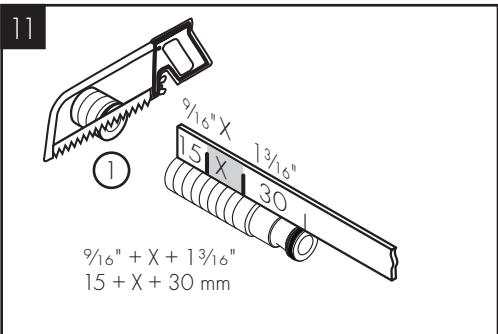
Cut the connecting thread so that it is  $X + 1\frac{3}{4}$ " ( $X + 45$  mm) long.
