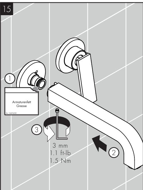
Lightly lubricate the o-ring on the connection thread.
