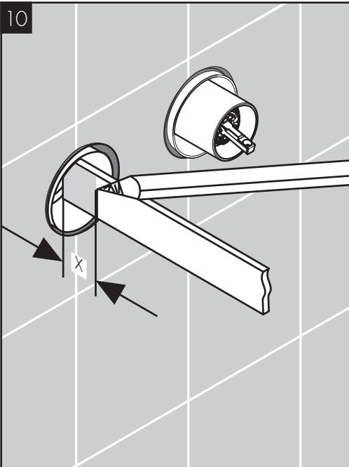
Measure the distance from the surface of the spout port rough to the outside edge of the plaster shield ("X").
