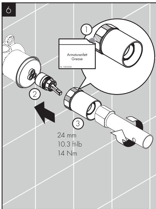
Lightly lubricate the threads on the nut.
