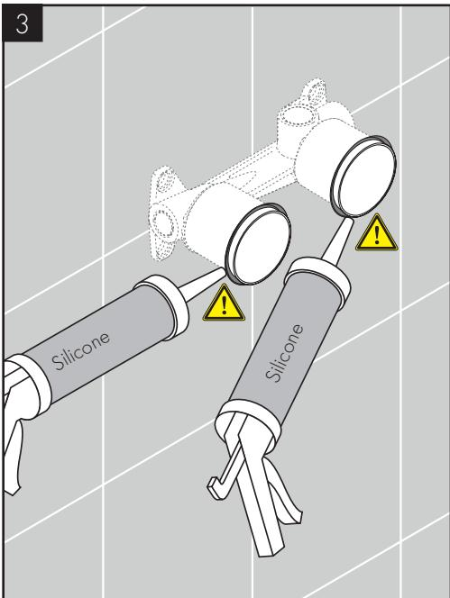
Seal the wall around the plaster shields using water-proof sealant.
