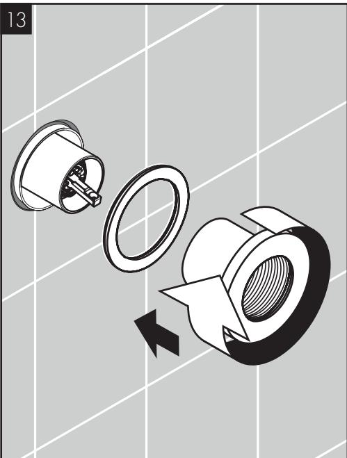
Install the washer and the sleeve/escutcheon assembly over the cartridge.
