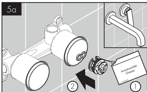
Lightly grease the o-ring on the cartridge adapter.
