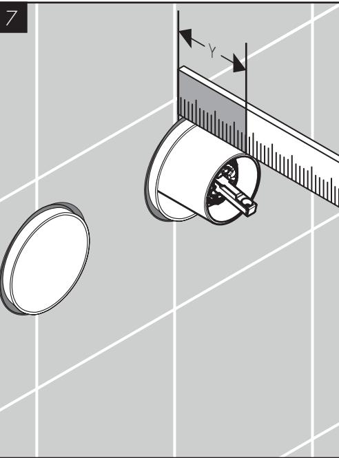
Measure the distance between the wall and the top of the nut ("Y").
