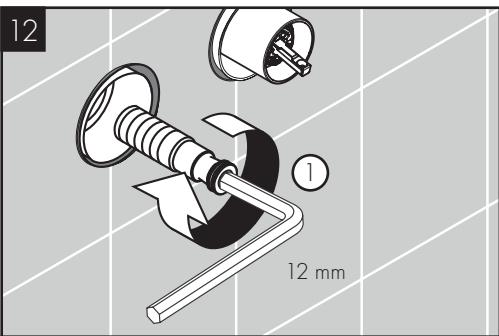
Install the connecting thread in the rough using a 12 mm Allen wrench.
