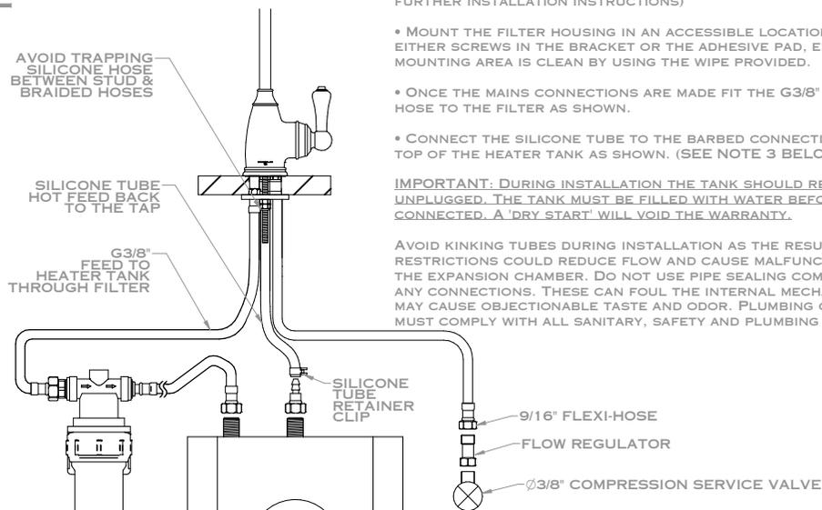
CONNECTIONS TO THE FILTER (U.1106) AND HEATER TANK U.1998: (SEE SEPARATE FILTER GUIDE AND HEATER TANK INSTALLATION FOR FURTHER INSTALLATION INSTRUCTIONS)
