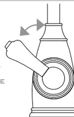
ONCE FINISHED, RELEASE THE HANDLE AND THE VALVE WILL AUTOMATICALLY CLOSE.
