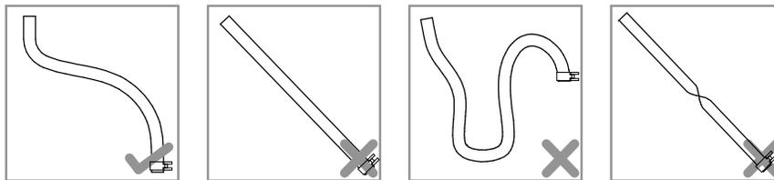
TRIM THE SILICONE HOSE TO THE RIGHT LENGTH FOR THE INSTALLATION. IT MUST NOT BE PULLED TAUGHT, TOO SLACK LEADING TO A 'U' BEND OR TWISTED. PLEASE MAKE SURE THE TUBE ISN'T PINCHED BETWEEN THE THREADED STUD AND THE BRAIDED HOSE AS THIS MAY CAUSE FLOW RESTRICTION. IF THE SILICONE IS NOT INSTALLED CORRECTLY IT MAY AFFECT THE PERFORMANCE OF THE SYSTEM.
