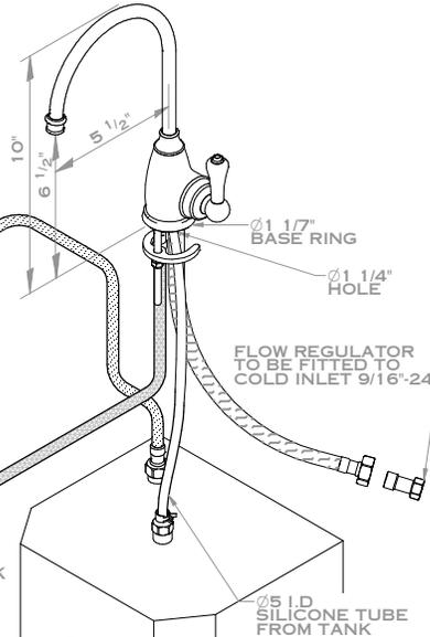
NOTE: DIAGRAM SHOWS FAUCET SET UP WITH U.1998 (HEATER TANK) AND U.1106 (FILTER).
